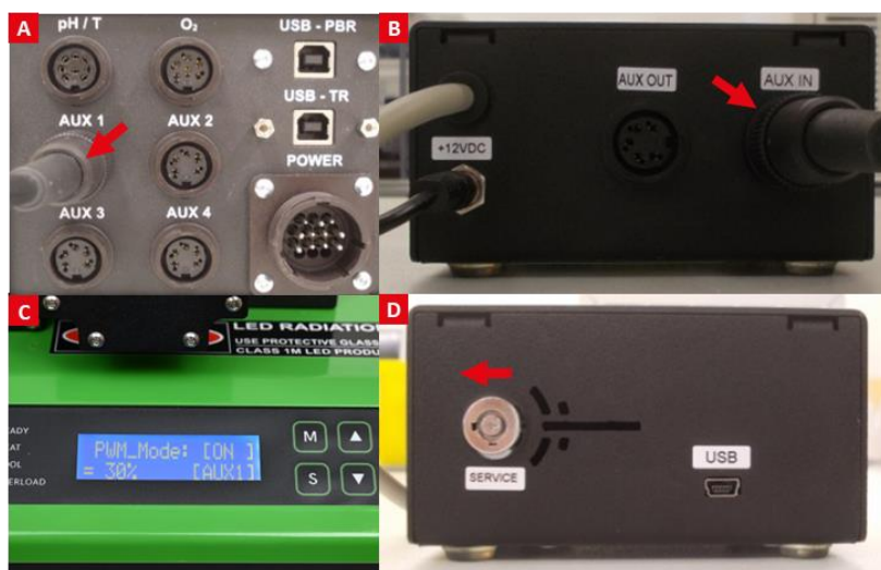
Fig. 29 Attaching of the AUX cable (A, B) and manual control (C) of magnetic stirrer.
