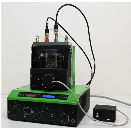
Fig. 28 Magnetic stirrer is fastened in the correct position to the front part of the PBR.
