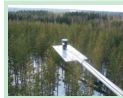
Skye 2-channel sensors on an Eddy-Covariance Tower. Courtesy: Dr Caroline Nichol
