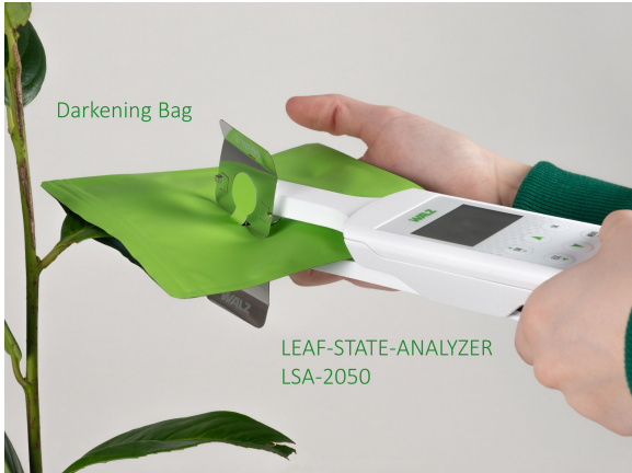
Probing a leaf after predarkening in a Darkening Bag (LSA-2050/DB). Dark acclimation is important for correct determination of the maximum Photosystem II yield, F_v/F_M .
