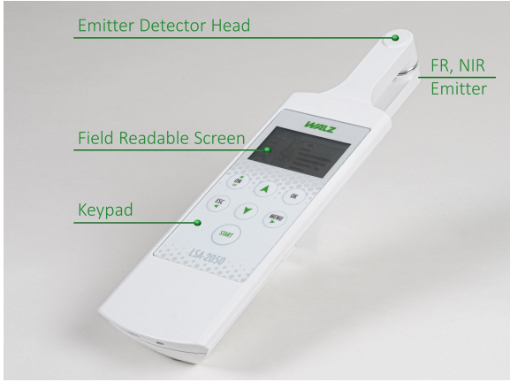
Functional units of the LEAF-STATE-ANALYZER LSA-2050. "Emitter Detector Head": LEDs and detector for screening and F_v/F_M measurements. "FR, NIR Emitter": LEDs for determination of chlorophyll concentration.
