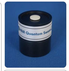
Measures Photosynthetically Active Radiation Counts quanta of photons in µmol m<sup>2</sup> s<sup>-</sup> Ideal or square PAR spectrum response For plant and crop research Commercial horticulture applications Suitable for natural and artificial light sources
